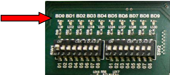
Figure 8 –BD0 to BD9 LEDs to indicate the communication rate
