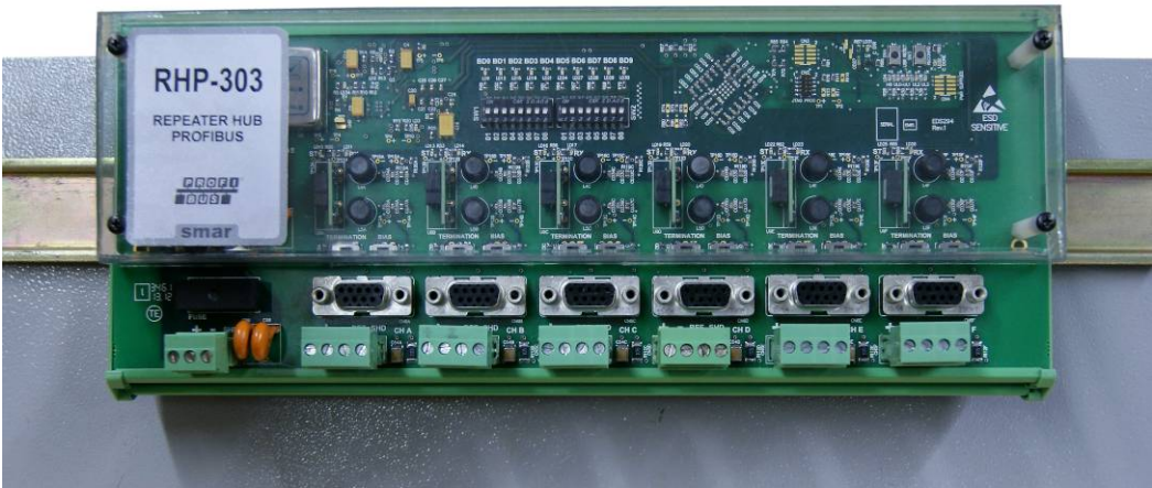
Figure 11 – RHP303 installed on a DIN rail
