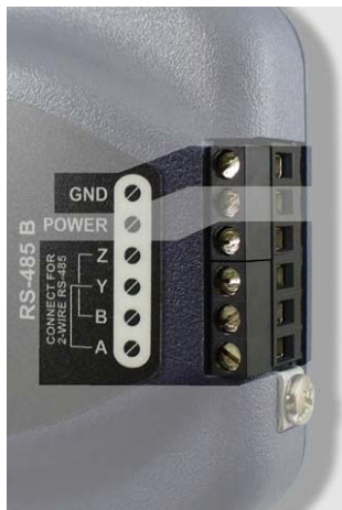
Figure 3: “RS-485 B” Terminal Block Network Connections
