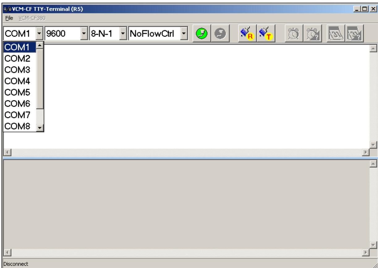
Communication Baud rate Setting: (2400bps / 4800bps / 9600bps)
