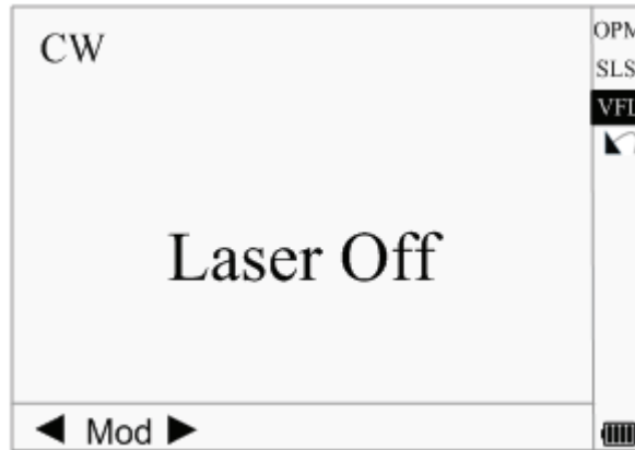
Figure 4-13. VFL Functional Interface
