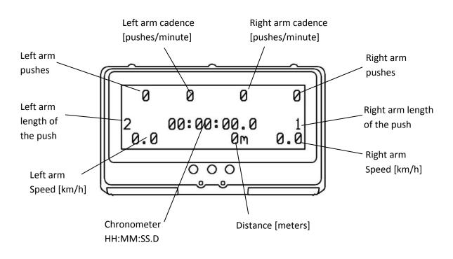
On this screen the middle button function as a reset of the number of pushes, distance and chronometer.
