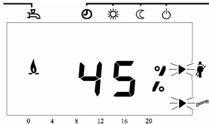
This mode allows burner heat output to be fixed manually
