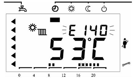
When a fault leads to boiler shut-down, a flashing display of the fault code replaces the boiler temperature display. An alarm bell is displayed in the bottom left corner of the display window.
