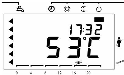
No heating demand has been received. The frost protection function is activated.
