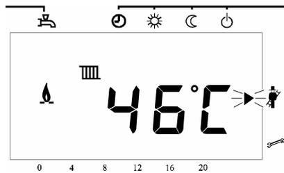
This mode allows the burner to operate at full load. Press and simultaneously for approximately 3 seconds
