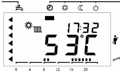
The regulator alternates Comfort and Eco modes, according to the time programming.
