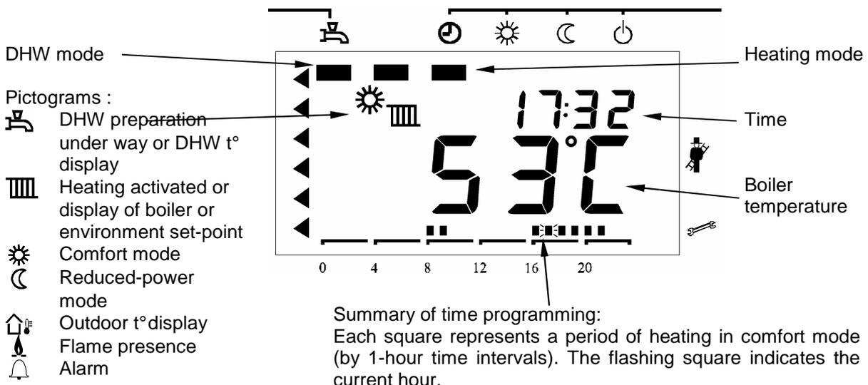
If a non-blocking fault occurs, the time display alternates with display of the fault code.
