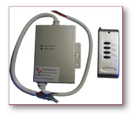
RGB Controller-S is specially designed for controlling LED multicolor changing patterns. Ist slim and delicate shape enables a no-sweat installation. The design flexibility on LED fittings will be enhanced enormously. The wireless controlling system is make your home decoration possible with industrial products.
