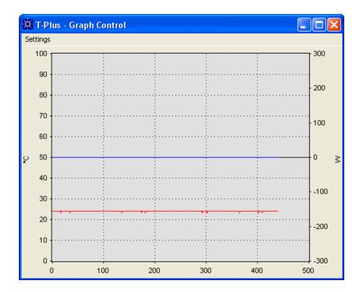
The Graph window plots till 8 different tracks allocable on two different Y axes and continuously shows their timing trend on the screen. You can add new fields right-clicking on the window list in the Single Pump Control Panel Window. The Graph window is completely sizable and it has axes limits completely configurable. Moreover for each track you can choose colour and Y axis (primary or secondary).
