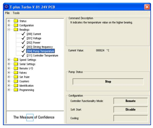
By this window you have the complete control of every pump (one a time) you find in the pumps list in the Main Window and here you can change or see pump settings, check status and parameters, configure a log or a plot and obviously give commands.
