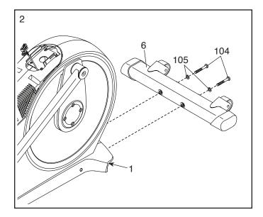
With the help of a second person, place some of the packing materials (not shown) under the rear of the Frame (1). Have the second person hold the Frame to prevent it from tipping while you complete this step.
