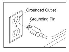
outlet must be on a nominal 120-volt circuit.
