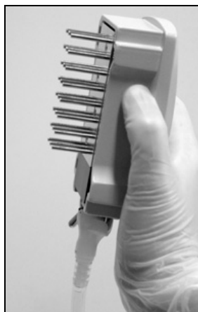
Figure 3. Illustration of the vacuum tool raised to beyond 90° vertical.
