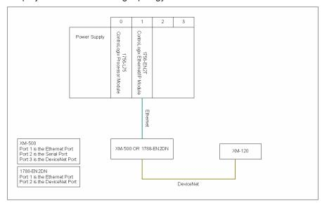
It uses an XM-500 module for the converter from Ethernet to DeviceNet. Even though the XM-500 can be a scanner module on DeviceNet it is not used as a scanner.
