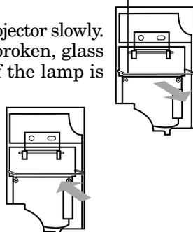
6. Insert the new lamp securely into the projector body in the right direction.
