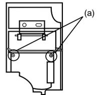
7. Tighten up the screws (a) using a phillips screwdriver (+).
