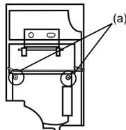
4. Loosen screws (a) using a phillips screwdriver (+), and remove them.
