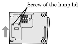
• Remove the lamp cover in the direction of the arrow as indicated.
