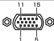
(Pin assignment of Mini D-SUB 15P jack)
