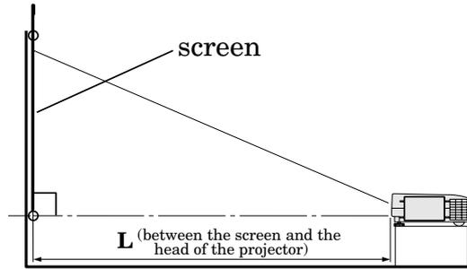
To find the approximate distance between the projector and screen: Multiply the width of the screen  $\times 1.9$  (min.), Multiply the width of the screen  $\times 2.4$  (max.).
