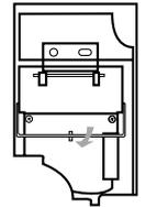
9. Tighten up the screws of the lamp lid using a phillips screwdriver (+).
