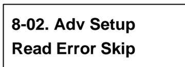
Press **ENT** to see the following figure. The default is Off. Press ▼ to select On.
