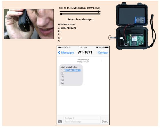
You already finish the set up. Now, you can use your mobile phone call to the SIM Card number switch the device on permanently. Another call to the SIM Card will switch the device off permanently.
