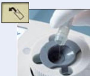
The Analyzer automatically senses the liquid and the intermittent beep continues for up to 20 seconds while the instrument takes a reading.
