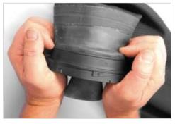
**1a.3** Press the Suit Ring evenly onto the seal so that the seal tightens in between the rings. Check for creases on the seal as creases may cause leakage.
