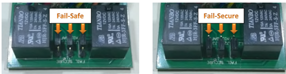
Figure 10: Fail-Safe and Fail-Secure Internal Jumpers
