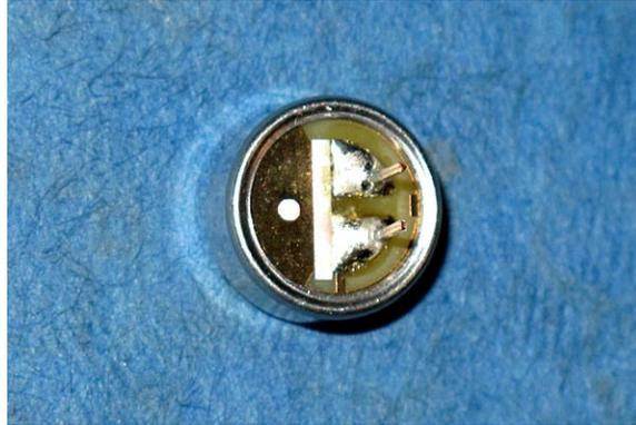
Figure 1: Back of the electret microphone. In this orientation, the lower terminal is “Terminal 2”, which should be connected to ground, and the upper terminal is “Terminal 1”, which should be connected via a series resistor to the positive voltage source (or terminal 2 to the positive power rail, and terminal 1 via a series resistor to ground).
