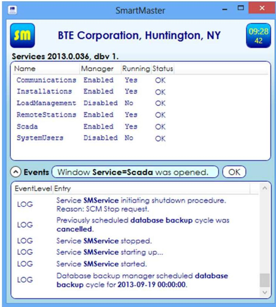
Each window is associated with one of system objects (subsystems) being monitored. In above case the window is associated with SmartMaster™ service, the top service, as described in previous section.
