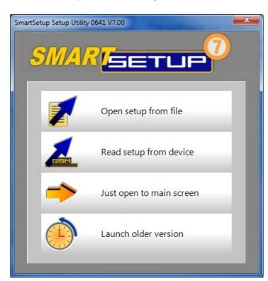
The software will show this screen when started. Here you can select whether you would prefer opening an existing setup from a file on your PC, retrieve the setup currently on the Micro Commander, just open to the main screen or launch an older version of the software.
