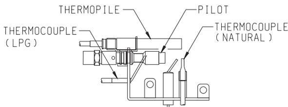
7. With the control knob pushed in, repeatedly push the piezo ignitor button until pilot is lit (or use a match to light pilot).
