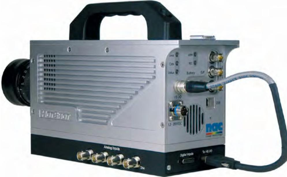
The Multi-Channel Wave Inserter (MCWI) connects to the camera via the High Speed Serial IO port. It has FOUR (4) analog and Sixteen (16) digital Channels. The sampling rate is determined by the FPS used on the camera and can be as many as 40 samples PER frame Period.
