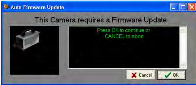
To proceed with the Firmware Upgrade you should press OK. If you CANCEL the process at this stage then the camera may not function correctly. In most cases, unless instructed otherwise by a NAC engineer, you should press OK.
