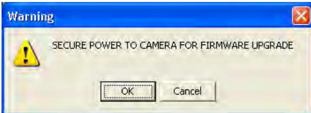
At this point you **MUST** make sure the power to the camera is secure. If you are using BATTERY power you should **NOT PROCEED** with the upgrade and should restart the process using MAINS power.
