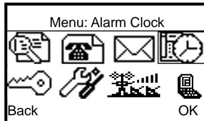
Use the navigation keys to highlight “Alarm Clock” in the main menu interface and then press “OK” to enter the “Alarm Clock” menu, the LCD will display:
