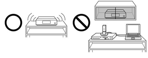
Adjust the location (height, orientation, and place in the room) of S-AIR products until reception is the most stable.
