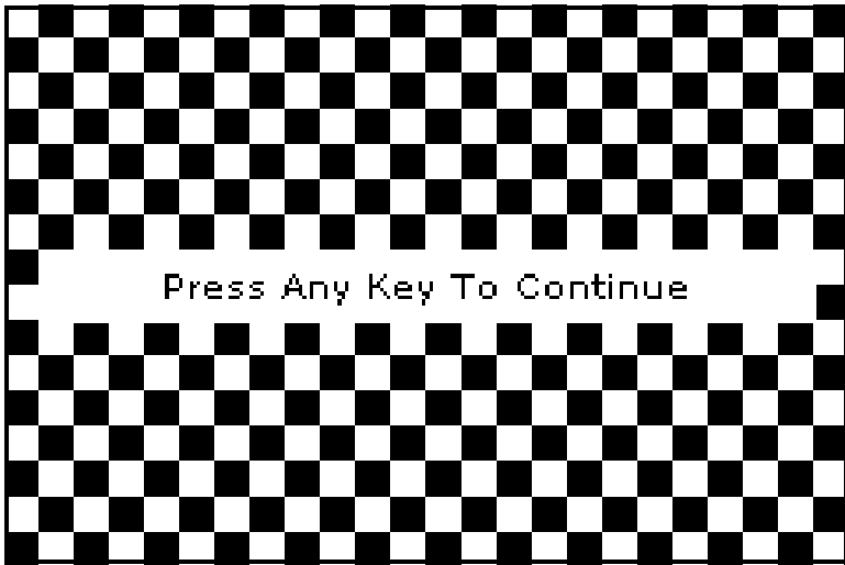
Figure 9-21: A Functioning Test Screen
