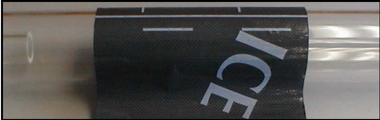
Figure 3-23: DMP-1 Dampening Material Wrapped Around Pipe
