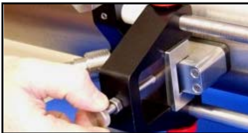
Figure 3-11: Installing the First Transducer
