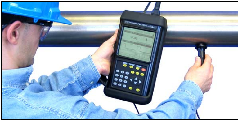
Figure 9-4: PT878GC Thickness Gauge in Operation
