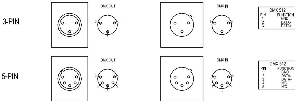
Connection between controller and projector and between one projector and another must be made with 2 core-screened cable, with each core having at least a 0.5mm diameter. Connection to and from the projector is via cannon 3 pin (which are included with the projector) or 5 pin XLR plugs and sockets. The XLR's are connected as shown in the figure above.
