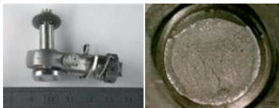
Broken part of actuator
