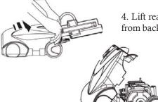
4. Lift rear latches up and tilt cover forward from back until front snaps free.
