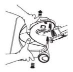
3. Turn brush over right side up. Press handle release pedal and lower the swivel. To remove cover, grasp the sides and pull out to release the outside cover.
