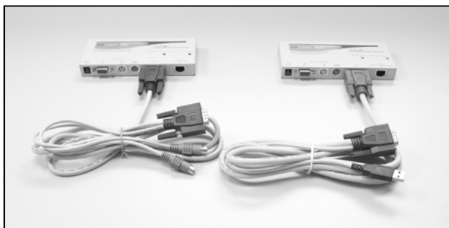
Figure 1: Connection of 3-in-1 and 2-in-1 cable
