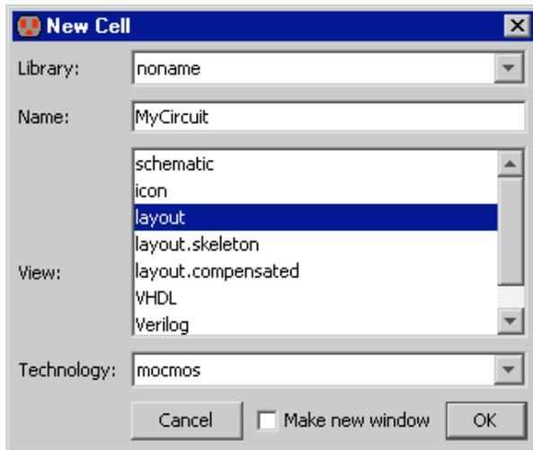
Before you can place any IC layout, the editing window must have a cell in it. Use the **New Cell...** command (in menu **Cell**). This will show a dialog that lets you type a new cell name. Type the name ("MyCircuit" is used here) and click OK. The editing window will no longer have the "No cell in this window" message, and circuitry may now be created.
