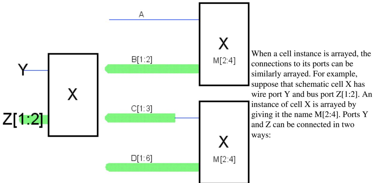
Implicit connection to all instances (top illustration). If the wire port Y is connected to a single wire (A), then wire A connects to port Y on all three instances of cell X. If the bus port Z is connected to a 2-wide bus (B), then each element of that bus connects to the same element of bus port Z on all three instances of cell X. So B[1] connects to port Z[1] and B[2] connects to Z[2] on all three instances, M[2], M[3], and M[4].
