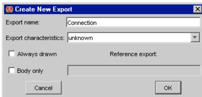
Move the cursor to the window with the lower-level cell ("MyCircuit") and select the contact node. Then issue the **Create Export...** command (in menu **Export**). You will be prompted for an export name and its characteristic (the characteristics can be ignored for now).
