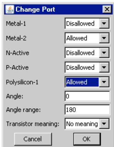
The other item that must be created is a port (more than one can be created, but for contacts, one is sufficient). Select the "PORT" entry from the menu on the left and place it in the display. You will be prompted for a port name, after which you can further move or stretch the port. Besides a location and a name, ports must specify which arcs may connect to them. To do this, double-click on the port.
