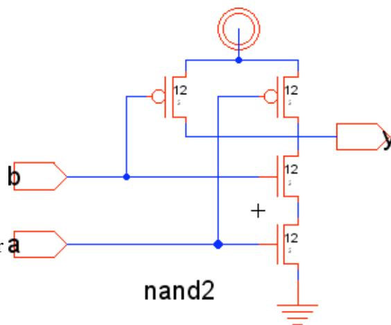
These symbols are *nodes* in Electric parlance. You may move the nodes around by clicking and dragging. The transistors default to a width/length value of 2/2. Double-click on the pMOS transistor and change its width to 12. Recall that nMOS transistors are roughly twice as strong as pMOS transistors. So a single nMOS transistor would only have to be 6 wide. However, because the nMOS transistors are in series, they should also be 12 wide.
