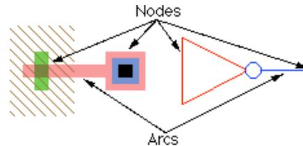
In the above example, the transistor node on the left has three pieces of geometry on different layers: polysilicon, active, and well. This node can be scaled, rotated, and otherwise manipulated without concern for specific layer sizes. This is because rules for drawing the node have been coded in a *technology*, which describes nodes and arcs in terms of specific layers.
