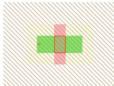
Although the default transistor is 2x3 in size, most people want them to be wider. For the purposes of this example, make the transistor be 12 wide. To do this, select the node and use the **Object Properties** command (in menu **Edit / Properties**).
