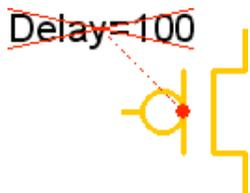
Note that text can be moved away from its attached node or arc. If this has been done, then selection of the text will also indicate the attached component by drawing a dashed line to it.
