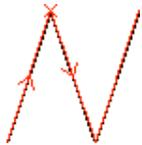
The Opened-Polygon node can be used to form the C-shaped body. When first created, it appears as a zigzag, shown here. To manipulate its shape, select it and enter "outline edit mode" by using the **Toggle Outline Edit** command (in menu **Edit / Modes / Edit**), or just type "y", or click on the icon in the toolbar.
