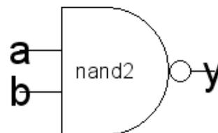
To edit the icon, click on it and use the **Down Hierarchy** command (in menu **Cell / Down Hierarchy**) or just type Ctrl-D. The Component tab will now show with various shapes (this is the "Artwork" technology). Delete the generic black box but leave the input and output wires. Turn on the grid.
