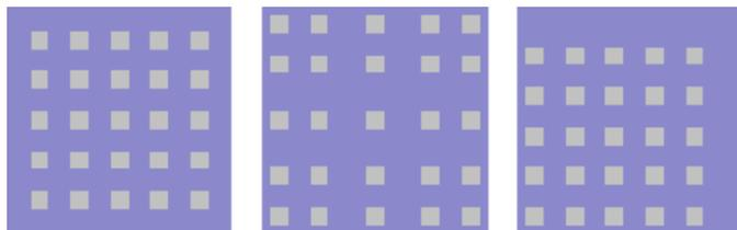
Contact nodes also have the ability to place the cuts according to different rules. The default (shown on the left) is to pack them as closely as possible in the center of the contact. Using the **Object Properties...** command (in menu **Edit / Properties**) you can change the "Cut Placement" to "At node edges" (the middle example) or "In node corner" (the rightmost example).
