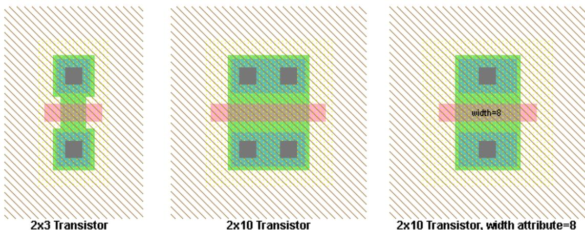
The scalable transistor on the left is 3 wide, and the other two are 10 wide. However, the scalable transistor on the right has the "width" set to 8, so it has shrunk.
