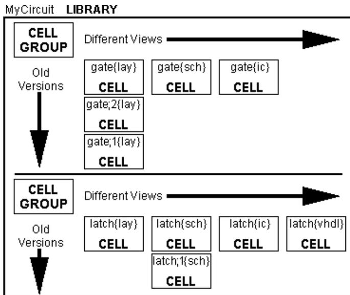
Besides organizing cells into a hierarchy, Electric also organizes cells into *cell groups* and gives each cell a *view* and a *version*. A cell's view describes its contents (for example "layout", "schematics", "netlist", etc.) A cell's version defines its design age. The full name of a cell is:
