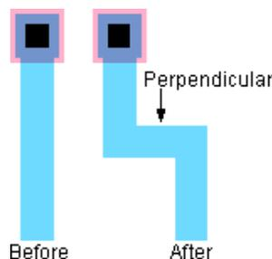
Once the jog is inserted, either half of the arc may be moved without affecting the other half, and the perpendicular arc will keep the circuit connected.
