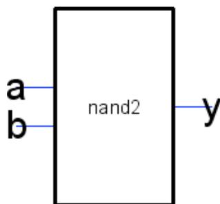
Edit your "nand2{sch}" cell and use the **Make Icon View** command (in menu **View**). Electric will create a generic icon based on the exports as shown here. It will drop the icon in the schematic for handy reference; drag the icon away from the transistors so it leaves the schematic readable.
