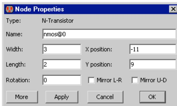
The dialog also has a field for the node's name. This name is not related to network information, but it must be unique, and can be used for identification. If a schematic node is given an arrayed name (such as "and[0:3]") then it indicates that the node is arrayed that many times. Nodes (and arcs) are automatically given unique names when first created (such as "nmos@0").
