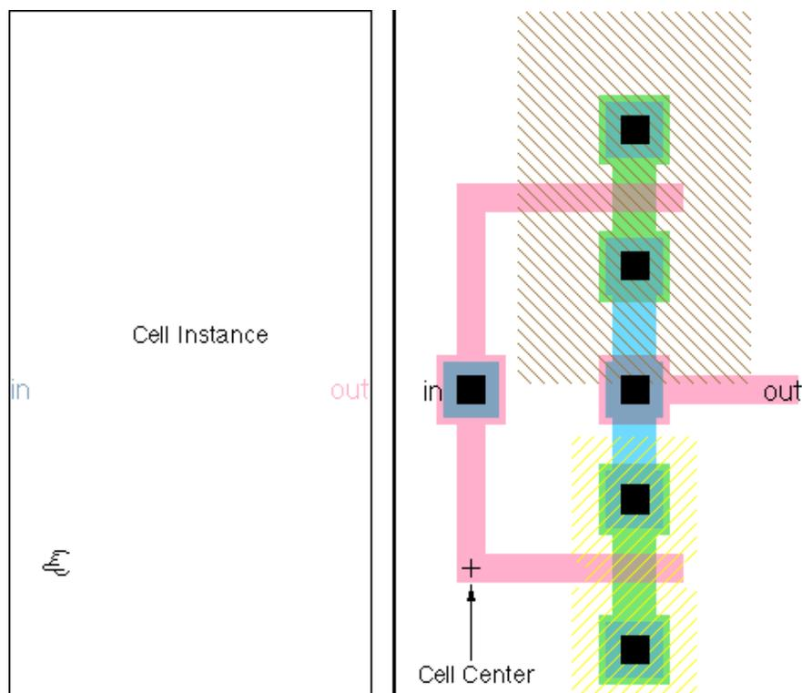
Most cells have a cell-center node placed automatically in them. If there isn't one and you want it, click on the "Misc" button in the component menu on the left, and choose "Cell Center". A cell-center node, placed inside of the cell definition, affects the anchor point for all subsequent creation of instances of the cell.
