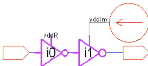
In the example here, two "invR" icons are placed, but only one of them has its "vddR" connection wired (to a different power source). The subcircuit for the rightmost icon will not use the global power signal, but will instead use the attached signal, "vddInv".
