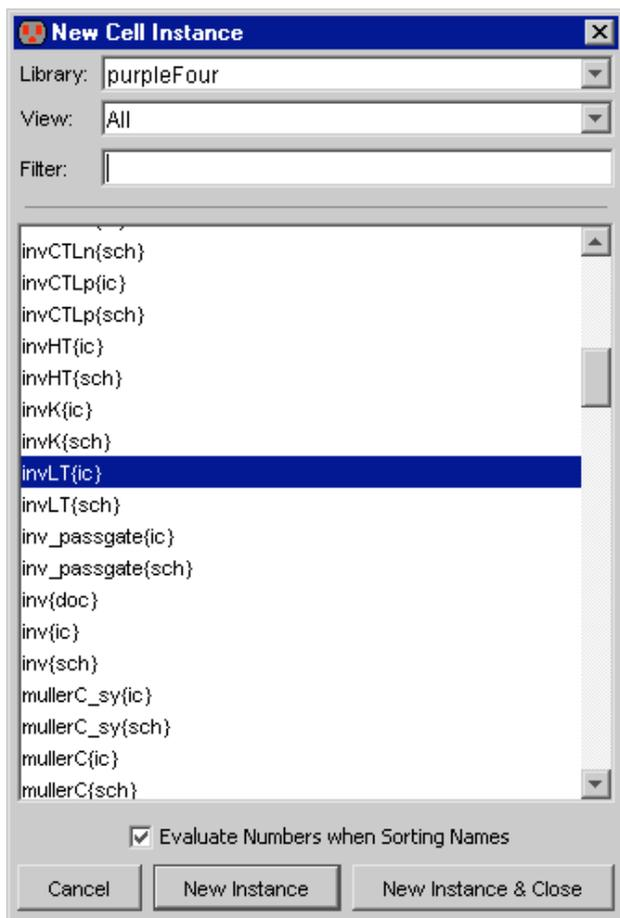
Another way to place an instance of a cell is to use the **Place Cell Instance...** command (in menu **Cell**). You will be shown a list of cells that are available for creation. After selecting one, click to create an instance in the current cell.
