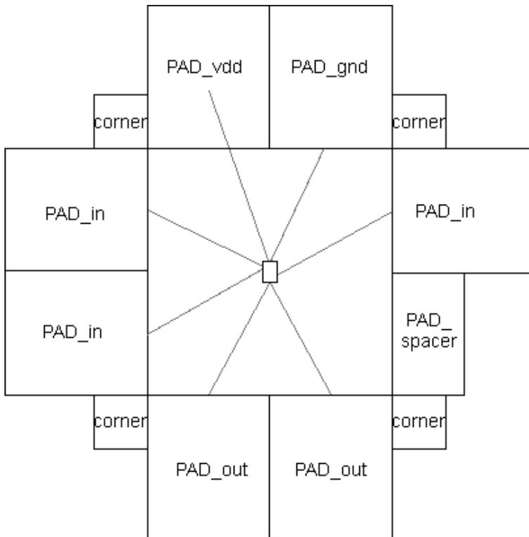
This file places 8 pads in a ring (2 on each side) and also places corner "pads" for making bends. The input pads connect to the 2 input ports "a1" and "a2". The output pads connect to the 3 output ports "out1", "out2", and "out3". The power and ground pads connect to the "vdd" and "gnd" ports.
