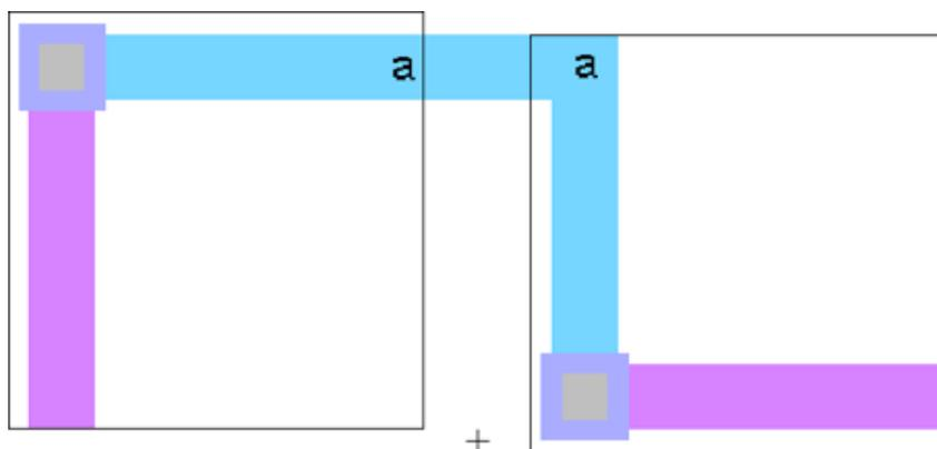
The top level of hierarchy (cell "high") has two instances of the cell "low" (the right instance is rotated 90 degrees) and an arc connecting them, as shown here.
