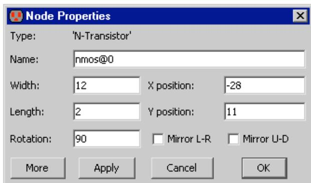
Two easier ways to see the objects properties are to double-click on the node, or select it and type Control-I. When the "node Properties" dialog appears, make the width 12 and click OK.
