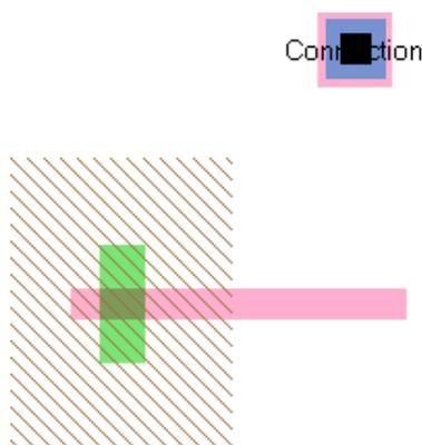
This takes the port on the contact node and exports it to the outside world. Its name will be visible on the unexpanded instance node in the higher-level cell.
