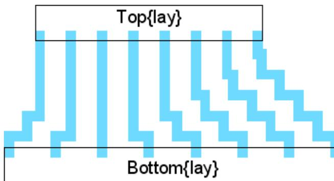
To specify an intended path for the river-router, every connection must be made with an Unrouted arc. Thus, before river-routing, there should be a series of direct (and presumably nonmanhattan) unrouted arcs. These arcs are replaced with the appropriate geometry during river-routing.
