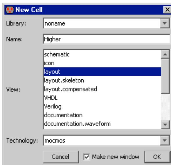
A new (empty) cell will appear in a separate window. Try creating a few simple nodes in this new window (place a contact or two).
