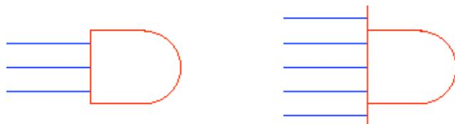
To negate an input or output of a digital gate, select the port or the arc and use the **Toggle Port Negation** command (in menu **Edit / Technology Specific**). With this facility, you can construct arbitrary gate configurations.
