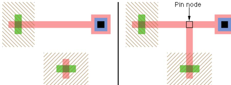
If it is sensible, the creation command actually uses one of the nodes on an end of the selected arc. However, if the connection falls inside the arc, it is split and a new node is created to make a "T" connection.
