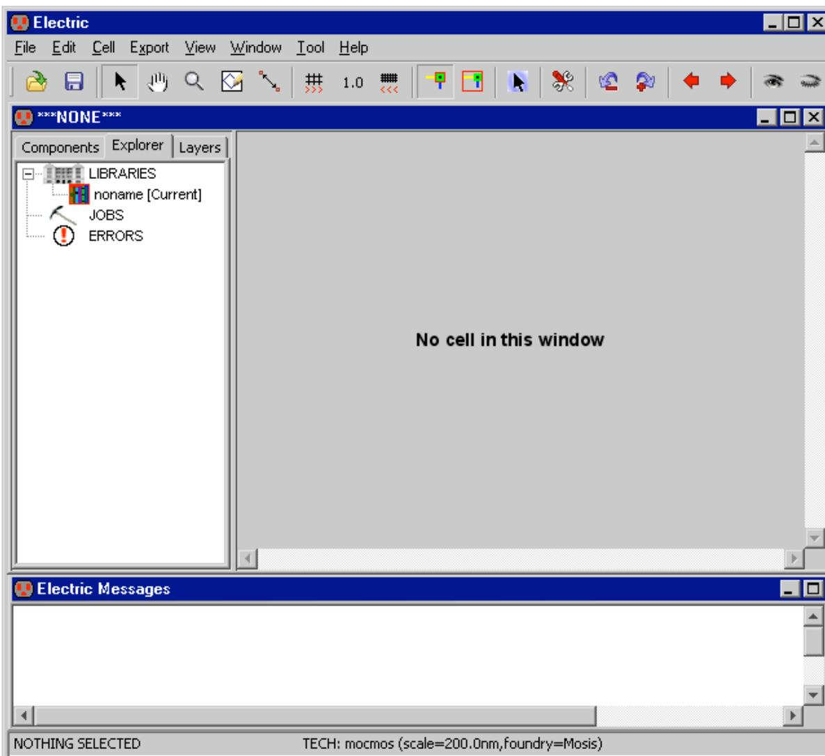
The *editing window* is the largest window that initially says "No cell in this window" (this indicates that no circuit is being displayed in that window). You can create multiple editing windows to see different parts of the design.
