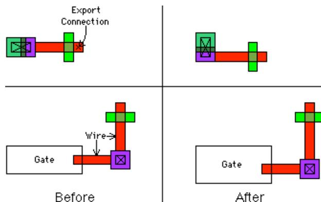
This bottom-up propagation of changes guarantees a correctly connected hierarchy, and allows top-down design. Users can create skeleton cells that are mostly empty and contain only exports on unconnected nodes. They can then do high-level design with these skeleton cell instances. Later, when circuitry is placed in the cells, or when layout views are substituted for the skeletons, the constraint system will maintain proper connectivity in all higher levels of hierarchy.
