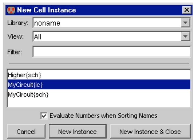
Now place an instance of the other cell by using the **Place Cell Instance...** command (in menu **Cell**). You can also click the "Cell" entry in the component menu. You will be given a list of cells to create: select the one that is in the OTHER window (the one called "MyCircuit{ic}" in this example). Then click in the newer cell to create the instance.
