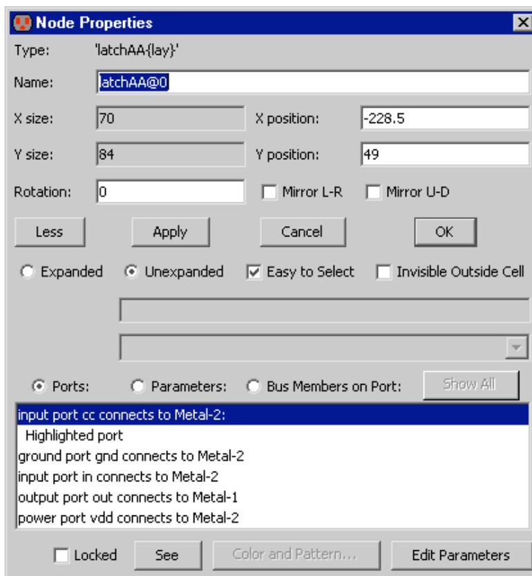
"Expanded" and "Unexpanded" control how the node is drawn (if it is a cell instance). An expanded instance is one that shows its contents; an unexpanded instance is drawn as a black box (see Section 3-4).
