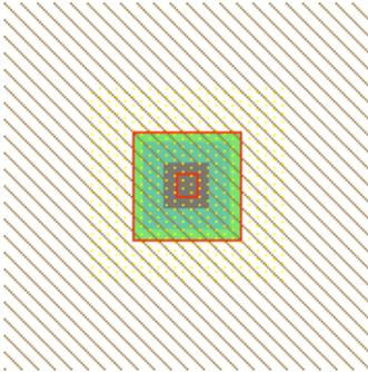
Next we need a contact. Choose a "Metal-1-N-Active-Con" to connect the N-Active to Metal-1. Make its size be 5x12 instead of the default 5x5. Notice that contacts are "smart" about the cuts, and add them to fill the node. Note also that the port (the inner rectangle) grows with the node.
