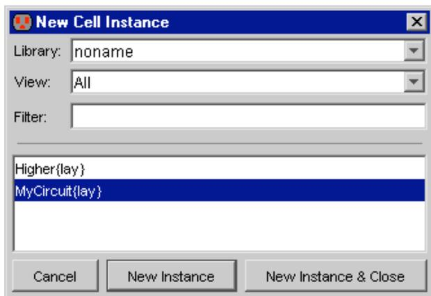
Now place an instance of the other cell by using the **Place Cell Instance...** command (in menu **Cell**). You can also click the "Cell" entry in the component menu. You will be given a list of cells to create: select the one that is in the OTHER window (the one called "MyCircuit" in this example). Then click in the newer cell to create the instance.
