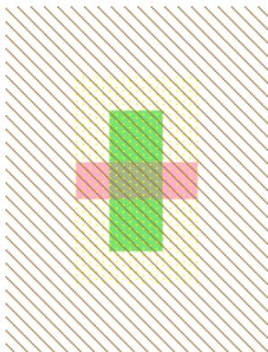
Start with a transistor (in this example on the left, an n-transistor). Rotate the transistor so that the gate is vertical. To do this, use the **90 Degree Counterclockwise** command (in menu **Edit / Rotate**), or just type Control-J. Note that the active gate on the left is highlighted (it is just a line).
