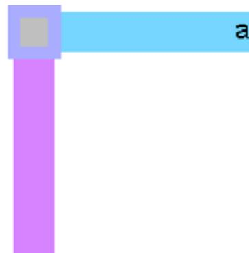
As an example of the JELIB format, let us assume a design with two levels of hierarchy. The bottom level of hierarchy (cell "low") has 3 nodes, two arcs, and an export, as shown here.
