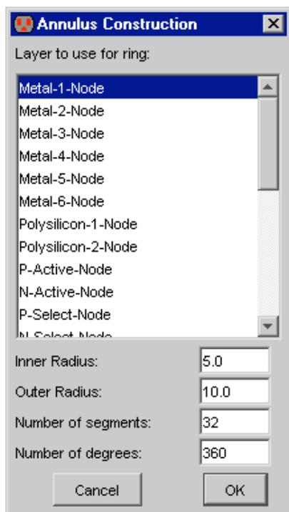
To generate a doughnut shaped outline, use the "Annular Ring..." command under the "Misc" entry in the component menu. This dialog prompts for a layer to use and an inner and outer radius for the annulus. By default, it is made as a full circle (360 degrees), but this can also be changed. Also, the number of line segments used in the construction can be set, allowing for smoother or coarser shapes.
