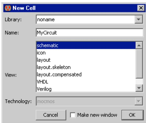
Before you can place any schematics, the editing window must have a cell in it. Use the **New Cell...** command (in menu **Cell**). Type the name ("MyCircuit" is used here) and select the "schematic" view.
