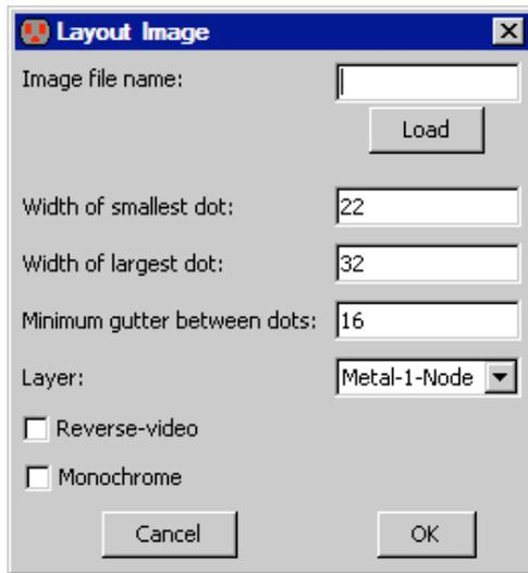
To generate images in layout, use the "Layout Image..." command under the "Misc" entry in the component menu. This dialog prompts for an image file and a layer to use as well as other factors in generating the image.
