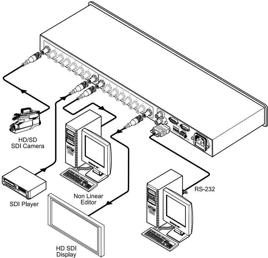
Figure 2: Connecting the VS-88HD 8x8 SD/HD-SDI Matrix Switcher
