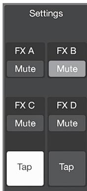
When an FX mix is selected, this area provides quick access to all FX mutes and Tap Tempo buttons for the delay effects.
