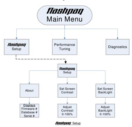
About: Displays Tuner Firmware Version, Database Version, Serial Number Set Screen Contrast: Allows changes to screen text & graphics darkness Set Screen BackLight: Allows changes to screen brightness level (Adjustable for extreme viewing situations – direct sunlight, nighttime, low lighting)
