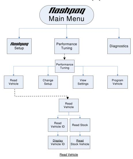
Display Vehicle ID: Displays vehicle identification from the connected vehicle Read Stock Vehicle: Reads the factory stock file(s) from the connected vehicle
