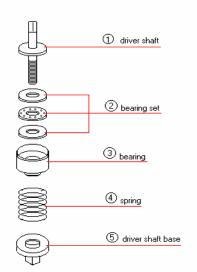
Lubricate #1, #2 & #5 as needed with molybdenum grease
