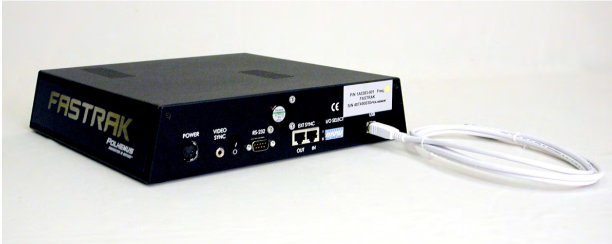
Figure 8-1 Connection of USB Cable to Switch to USB Mode
