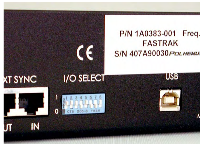
Figure 7-3 Default I/O Select Dip Switch Settings
