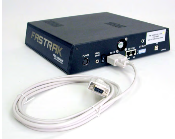
Figure 7-5 RS-232 Cable Connection
