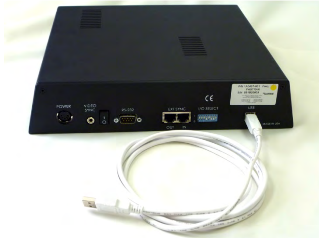
Figure 1-7 DC USB Cable Installation
