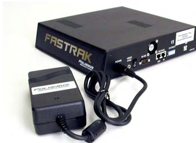
Figure 1-6 DC Power Cable Installation
