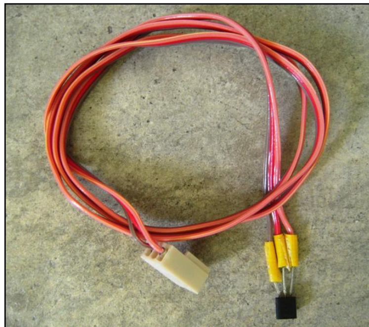
Figure 3.11: Rainbow wire used to connect LM35DZ with PIC MCU on SK40C
