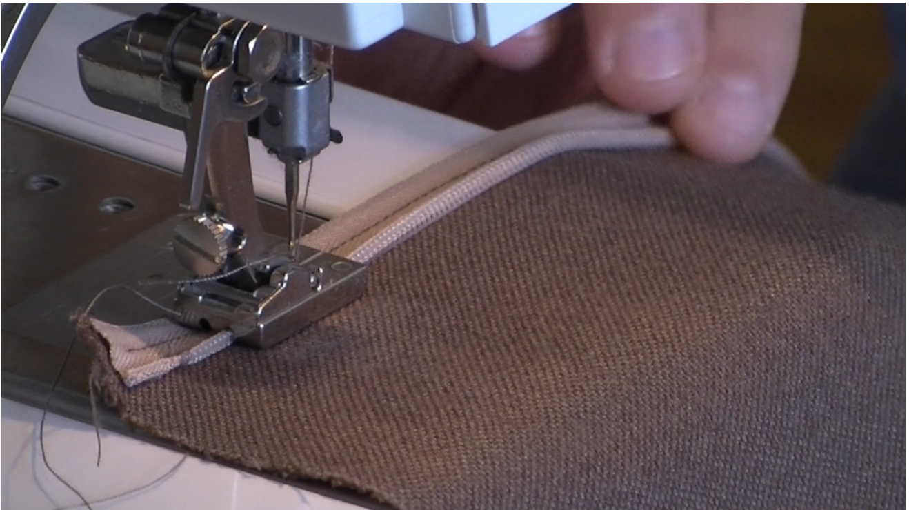
The concealed zipper foot will attach an invisible zipper into a garment with ease, it turns the coils of the zipper as the machine stitches creating a perfectly inserted zipper into a garment, a must have presser foot for the discerning sewer as many ladies garments are designed with the concealed zipper in mind
