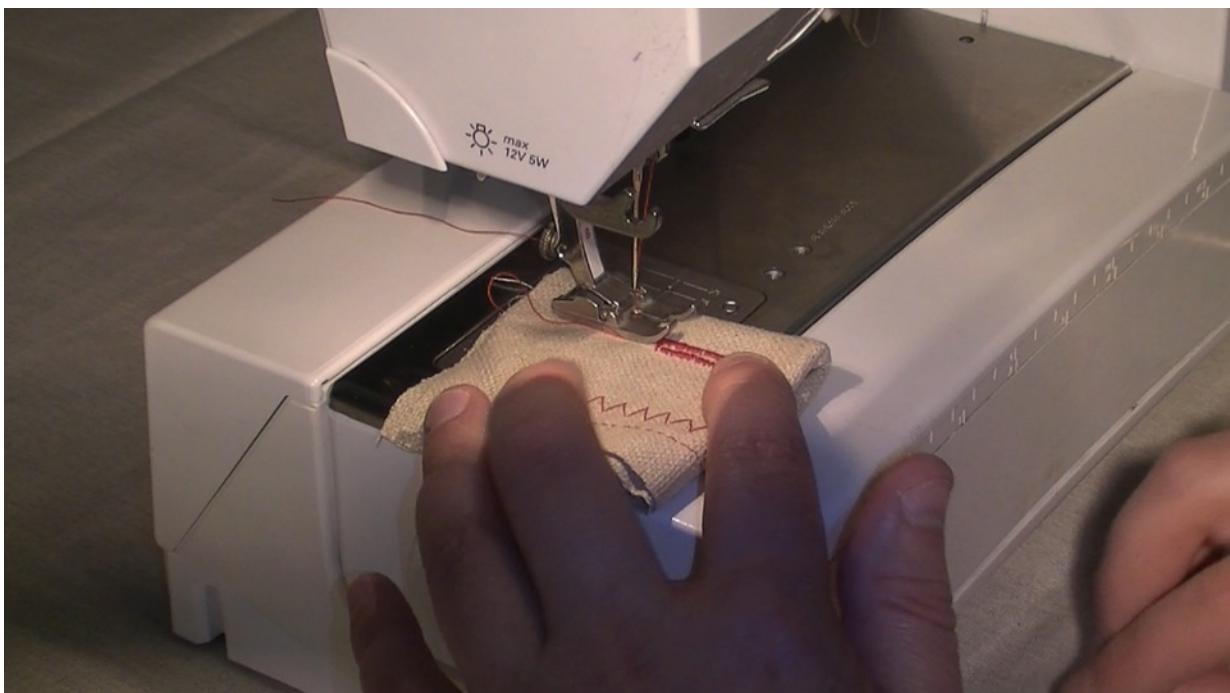
The thicker machine needle will penetrate many layers of cloth at once when the denim foot is attached
