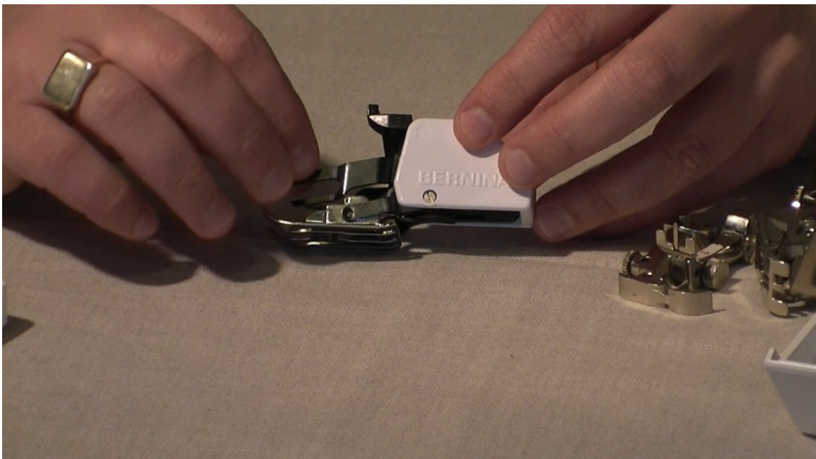
The walking foot, ideal for all sewing including leather and difficult to control fabrics
