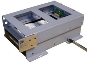
5. Put the HDD bracket back, and make sure to fasten the screws firmly.
