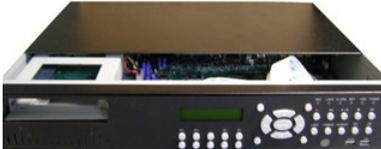
2. Disconnect the SATA cable & 4-pin HDD power cord.
