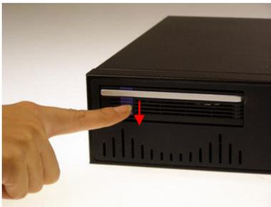
2. Pull the silver shaft forward slightly to the end, and the hot-swap tray will slide a bit.
