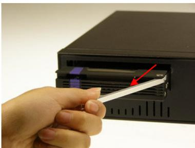
4. Install SATA HDD into the Hot-swap tray, and use screws to tighten it.
