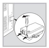
1 Open the terminal board by inserting a screwdriver into the side tabs of the cover. Use the
