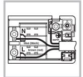
2 Loosen the cable clamp screw and remove it, using a screwdriver as a lever (see figure).
