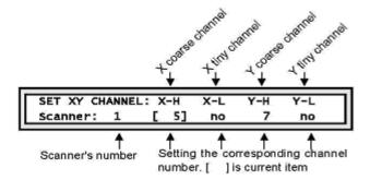
For 16Bit scanner, if the values of X-H, Y-H are set and the values of X-L, Y-L are set to [no], the 16Bit scanner will be running in 8Bit X/Y resolution. The will lost some characteristics of 16Bit scanner, such as high precision of X/Y orientation and the smoothness of the moving trace.
