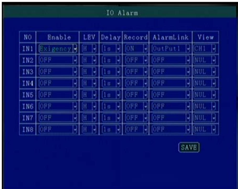
“Enable”:Alarm Trigger enable on/off and alarm type, press [OK] for changing;
