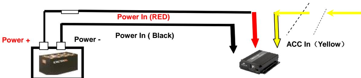
Red cable connect positive of the car battery, black cable connect negative,while yellow cable connect independent ignition switch or independent positive.
