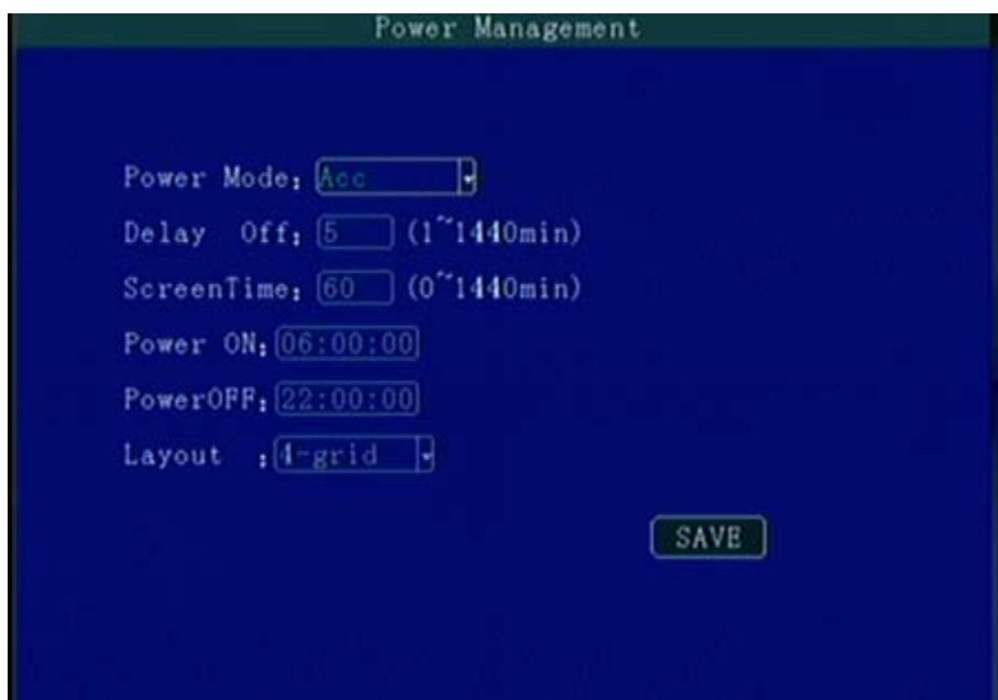
"Power mode": press the number keys to select the type, the default is ignition mode.
