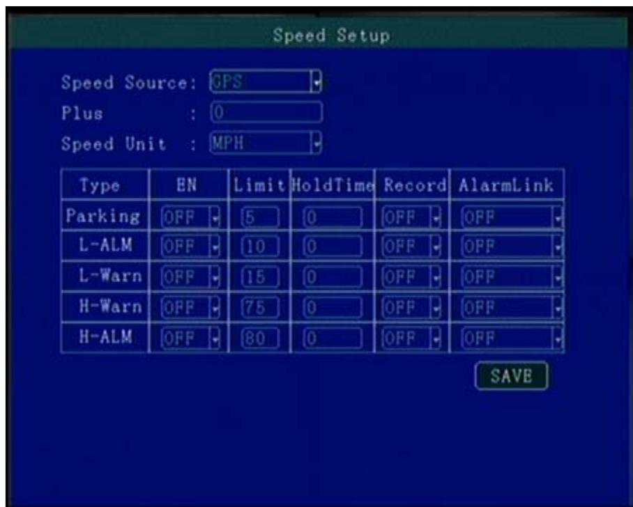
“ Speed Source”: The method to get speed, GPS/Pulse Signal Optional, Press [OK] for changing;
