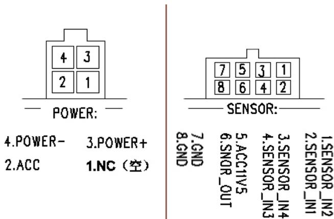
Among them, SENSOR\_IN\* is Alarm Input port; SENSOR\_OUT is Output Control port;
