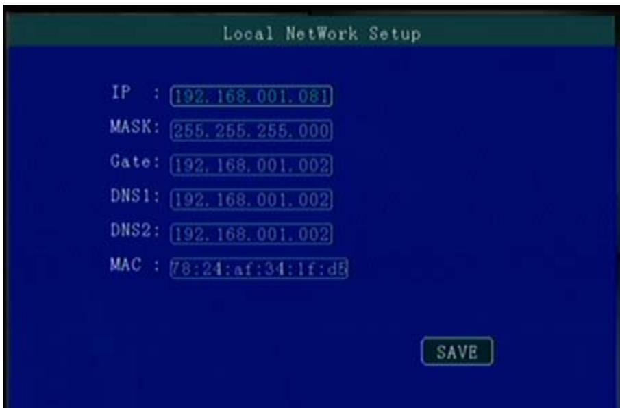
“IP”\“Mask”\“Gateway”\ “DNS1” \“DNS2”\“MAC”:IP,Mask,Gateway,MAC setting for LAN network testing,
