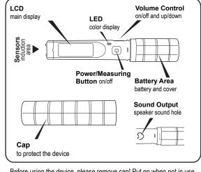
Before using the device, please remove cap! Put on when not in use to protect cap again!
