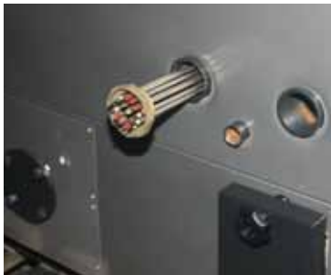
1. Installation of the resistance
