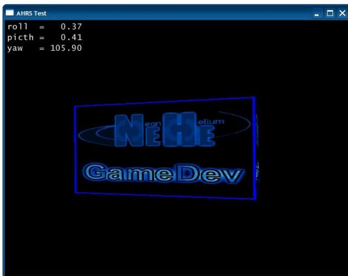
**Note:** the actual Refresh Rate of the data is related to Baud Rate, such as, if the Baud Rate is “19200”, while you want to set the Refresh Rate to “100HZ”.In this situation, even though you can set to “100HZ”, the actual Refresh Rate can’t reach 100HZ. Therefore, if you want a high Refresh Rate, you have to turn up the Baud Rate at first.
