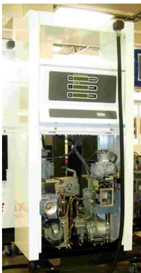
Figure 23 – Dispenser SDA 2222. without its cover,
