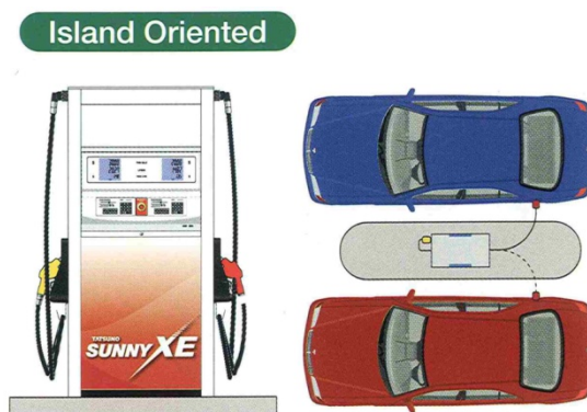
Figure 2 – Narrow double-sided dispenser with guns on its sides (NARROW, ISLAND ORIENTED)
