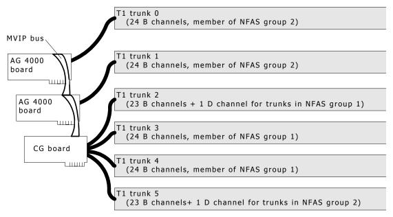
If your application uses NMS ISDN software in a channelized configuration, all trunks in an NFAS group must be on the same board. An NFAS group cannot contain trunks from multiple boards. This restriction does not apply to the ACU or LAPD configurations.
