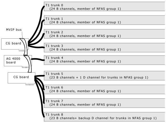
At any point in time, only one D channel conveys B channel signaling information. The other D channel remains in a standby mode and is only active at the LAPD layer (layer 2). While the backup D channel is on standby, any layer 3 messages received on it are ignored.
