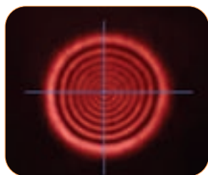
Figure 2: Make sure that the target is aligned with the pilot light. This must be checked every time the laser is used.
