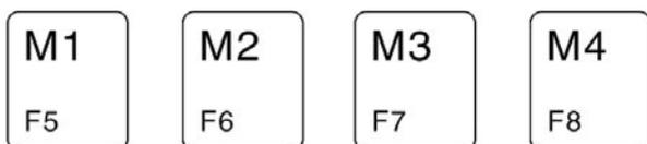
These keys are not assigned, which is why a circle with a line through it appears on-screen if you press one of the four keys. This symbol indicates that a function cannot be carried out.
