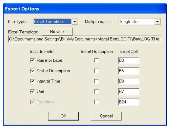
This screen is used to modify the default selections for the file type and run description fields to be exported from the Log Upload Display. When data is initially uploaded the selections are set to these default values. After the initial data display, the selections may be temporarily changed for each export operation, and remain changed for the duration of the data display. Logged temperature readings are always exported.
