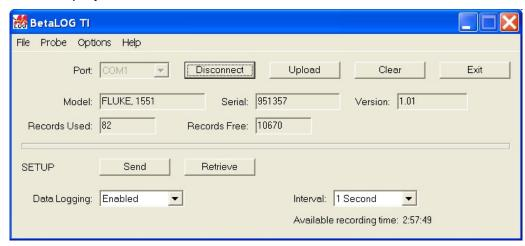
The top portion of the display contains controls to connect to a probe, disconnect from a probe, upload logged data, clear logged data, and exit the application. Once connected to a probe, it shows the model, serial number, and firmware version of the probe. The number of data logging records presently used and free is also displayed if data logging is enabled in the probe.
