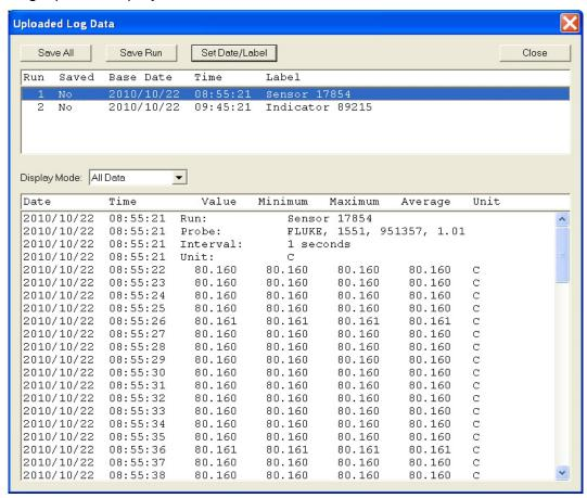
The top portion of the display lists the individual data logging runs found in the uploaded data. To display a run's data in the lower portion of the display, highlight it by clicking on it.
