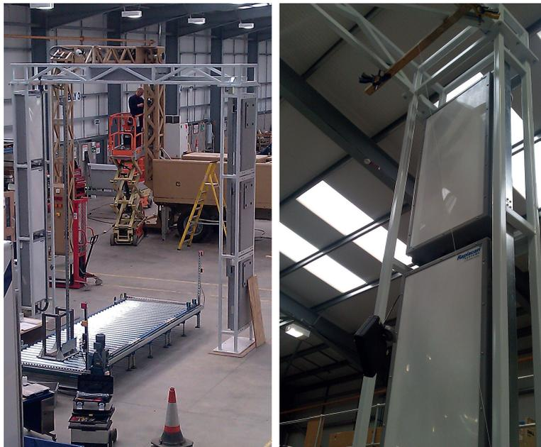
Figure 1.2: Picture of the Rad-Nuke Vehicle scanning Detector System
